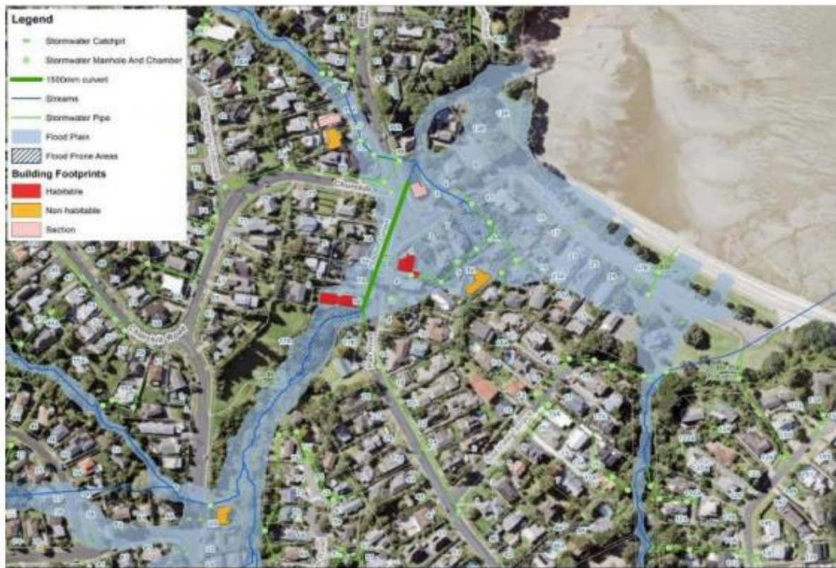
Figure 1 Flooded properties in the three storm events in 2018 at Cockle Bay (Reference 2)
